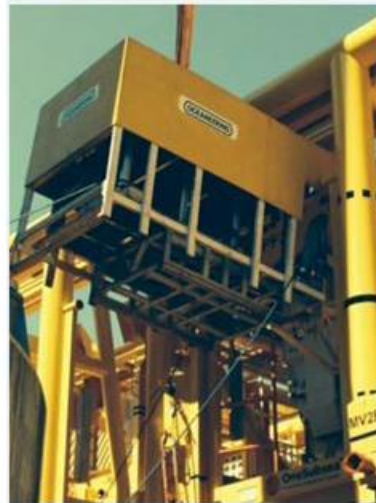
Mock-up ROV access test
