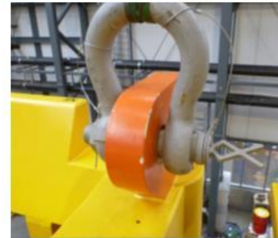
Test of Ocean Install shackle towards the Pump Station
